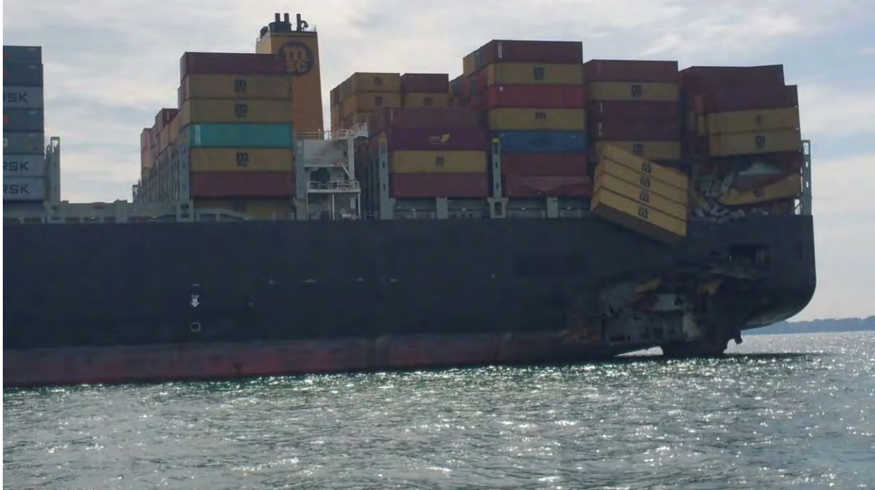
Collision damage to MSC Alexandra after impact with Dream II, 2016 (Image courtesy Rob Perkins / X)
