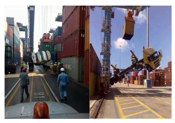
Lifting device operators, workers releasing chassis twistlocks and signal persons each have an obligation to work closely with one another <u>on every lift</u>, in order to ensure that the load is securely engaged before hoisting, and that container-carrying vehicles are not going up with the load.
